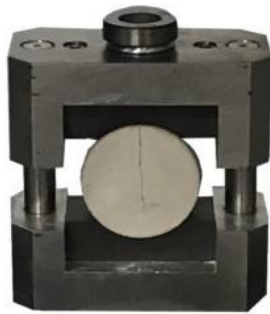
Standard ITB 250 (Max diameter: 76 mm)
